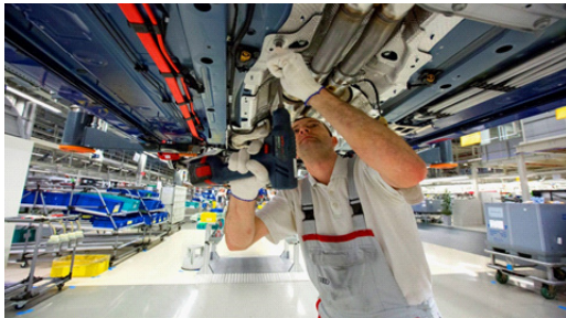
An employee bolts a heat shield to the undercarriage of an Audi AG car at the carmaker’s factory in Neckarsulm, Germany. Source: Bloomberg News
